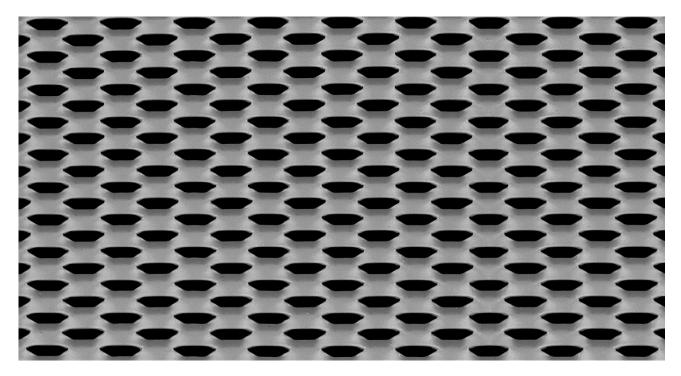
LW Pitch:19.05mmStrand Width:3.00mmSW Pitch:7.62mmThickness:0.60mmWeight:3.90 kg / m2Open Area:21%
